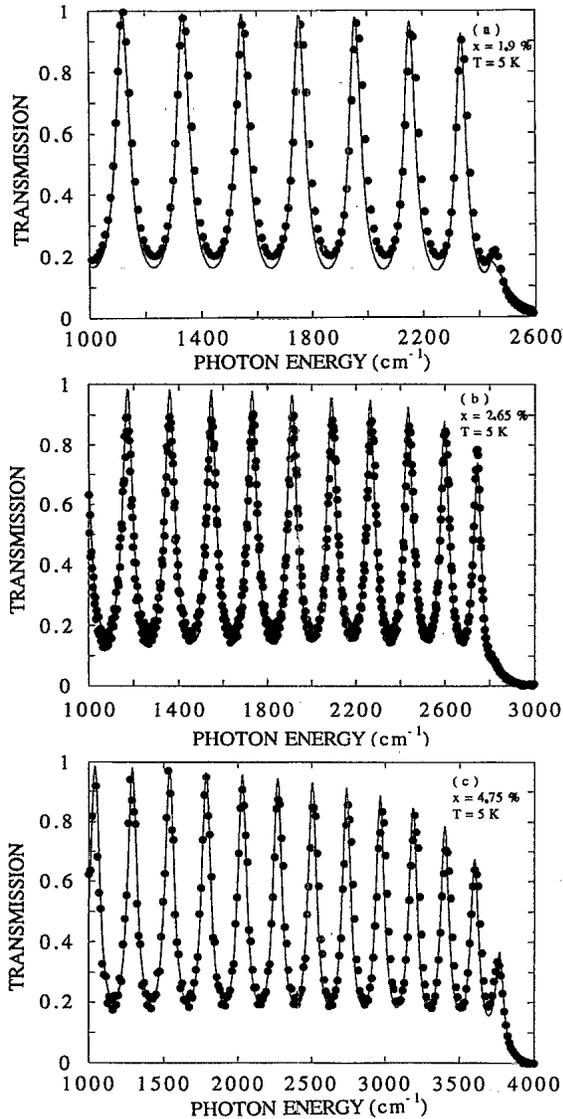
FIG. 2. Transmission spectra of Pb<sub>1-x</sub>Eu<sub>x</sub>Te epitaxial layers on BaF<sub>2</sub> at  $T=5$  K for various Eu contents: (a) sample B,  $x=0.019$ ; (b) sample C,  $x=0.0265$ ; (c) sample D,  $x=0.0475$ . The solid lines are model fits according to the nonparabolic two-band model.
