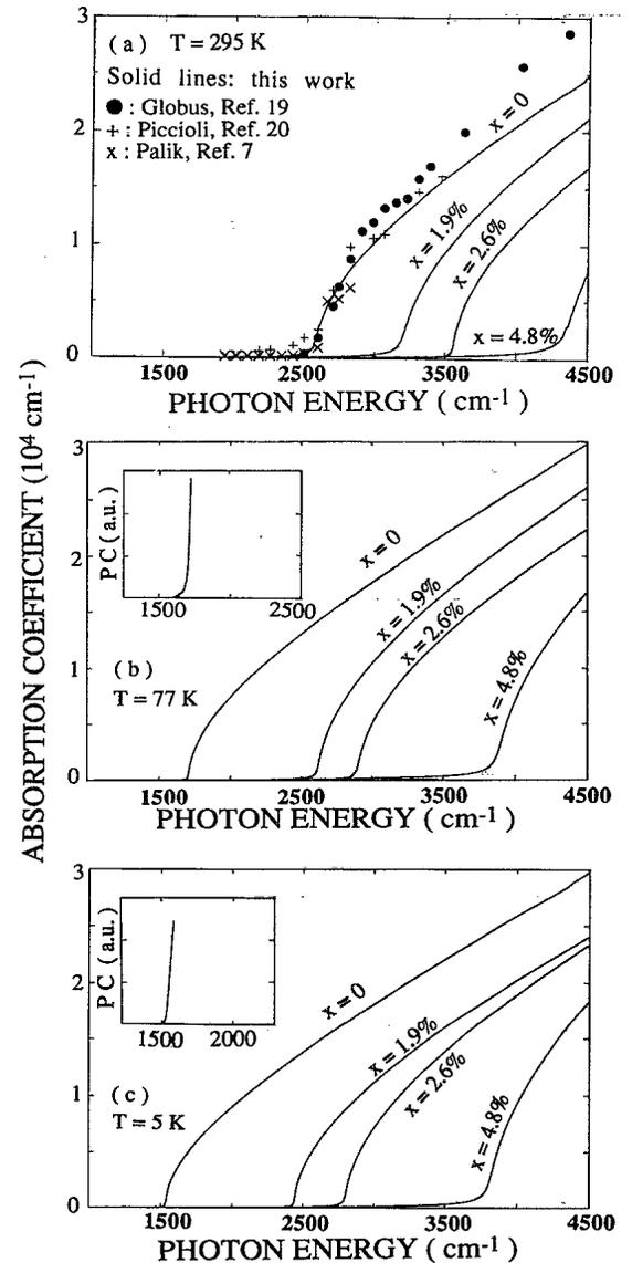
FIG. 3. Absorption coefficient  $\alpha(\omega)$  for PbTe (sample A) and  $\text{Pb}_{1-x}\text{Eu}_x\text{Te}$  (samples B, C, and D) at three temperatures: (a) 295 K, (b) 77 K, (c) 5 K. The insets in (b) and (c) show photoconductivity spectra (PC) which reproduce the onset of absorption in excellent agreement with fits to the transmission spectra.
