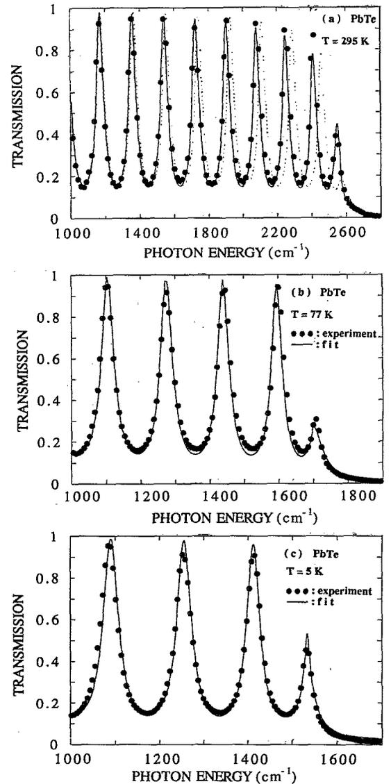
FIG. 1. Transmission spectra of a 4.5- $\mu\text{m}$  epitaxial layer PbTe on BaF<sub>2</sub>, sample *A*, for various temperatures: (a) 295 K, (b) 77 K, (c) 5 K. The solid and dashed lines are model fits: the best agreement with experimental data (circles) is obtained by using the nonparabolic two-band model (solid lines), whereas in the limit of a parabolic two-band model (with identical band-edge masses) the phase of Fabry-Perot interferences does not fit the measurements as shown in (a).
